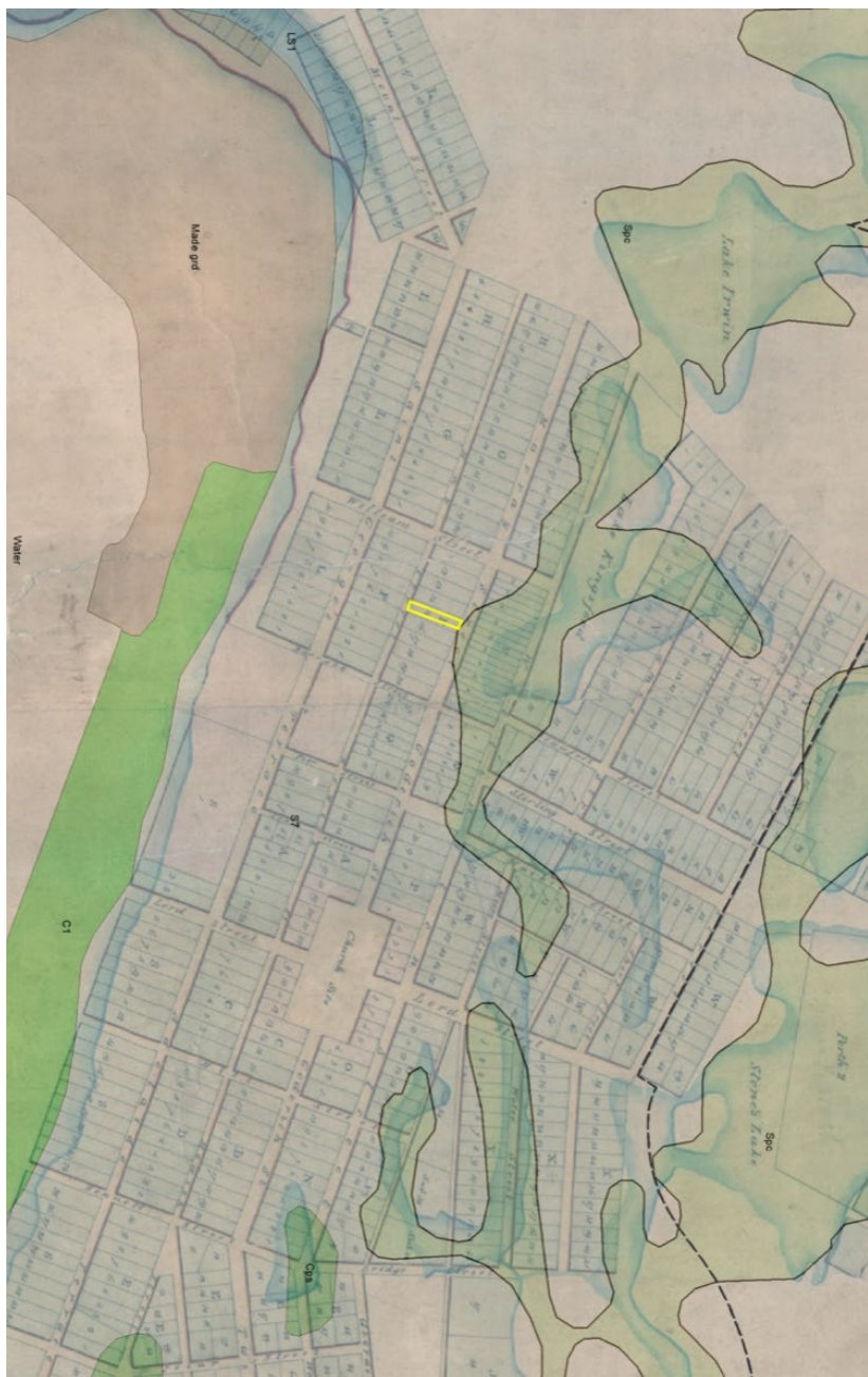
1838 map of the Township of Perth showing Kingsford Lake and Riverbank supported by geology, soil data, and vegetation complexes that respond to hydrology and elevation. The current location of Carillion City is marked in yellow, where peaty (SPC) and Karrakatta (S7) sands are likely present.
